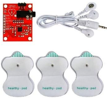
Fig 2. ECG signal acquisition kit AD8232
