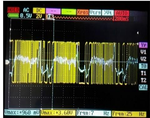
Fig 8.: Evolution of the modulated signal (ECG) and the modulated signal
